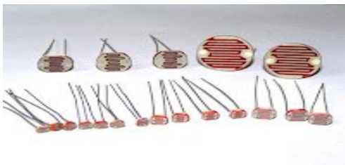
Gambar 2.16. LDR (Light Dependent Resistor)
